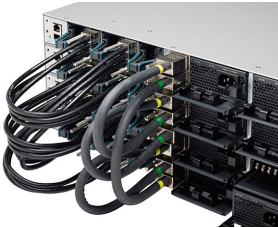
Figure 8. StackWise-480 and StackPower Connectors
